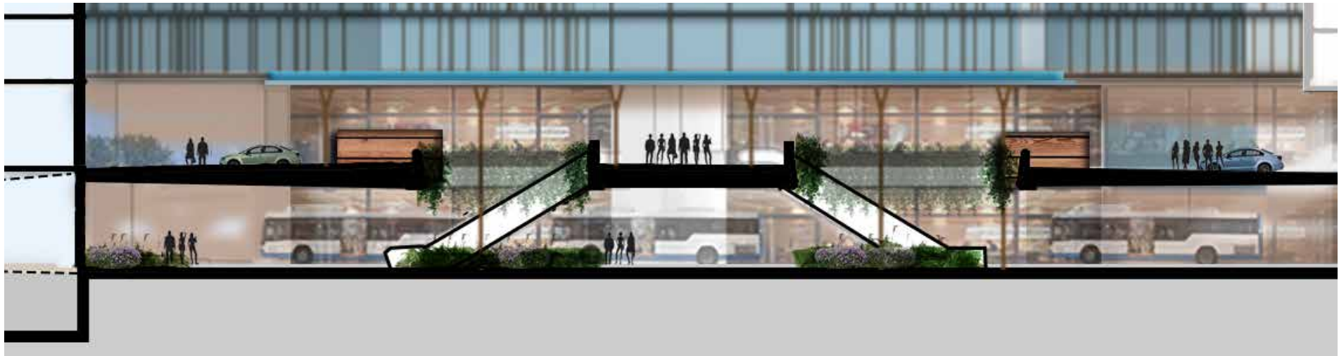
Vertical transportation provided between Levels 1 and 2 link the two levels of the bus terminus and plaza
