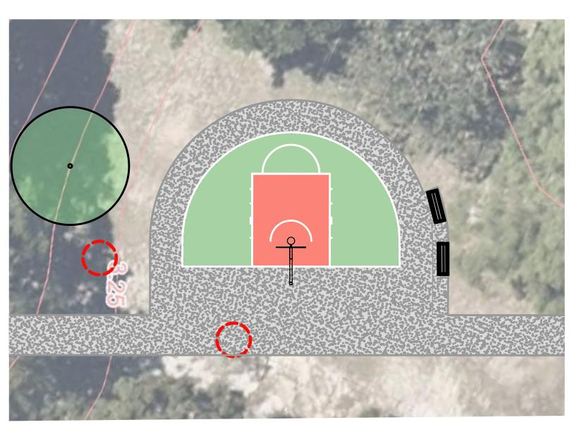
OPTION D - LINEMARKING WITH CONCRETE COURT SURFACE IN TWO COLOURS
